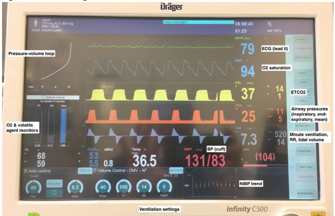
Figure 4: Labelled image of an anesthetic machine
